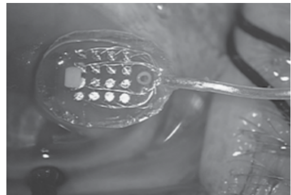
Fig. 4. Photograph of the Second Sight Model 1 epiretinal microelectrode array prior to insertion into the vitreous cavity in a patient with longstanding retinitis pigmentosa.
