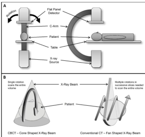
Fig. 1. (A) is a diagrammatic representation of a typical construct in a CBCT system. (B) is a diagram showing the difference in X-ray geometry of CBCT and conventional CT.
