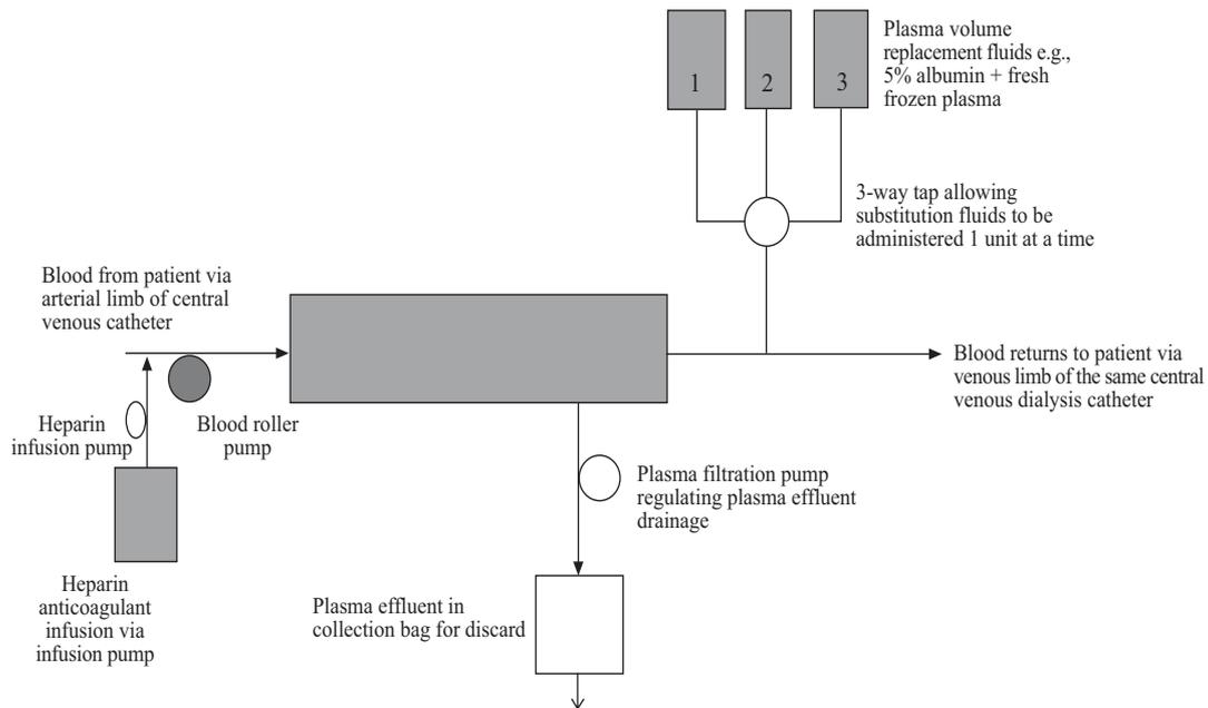
Fig. 3. Diagrammatic representation of standard membrane plasma filtration (PF) extracorporeal blood circuit.
