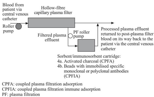
Fig. 4. Diagrammatic representation of (a) coupled plasma filtration adsorption (CPFA), and (b) coupled plasma filtration immunoadsorption (CPFIA) extracorporeal blood circuits.
