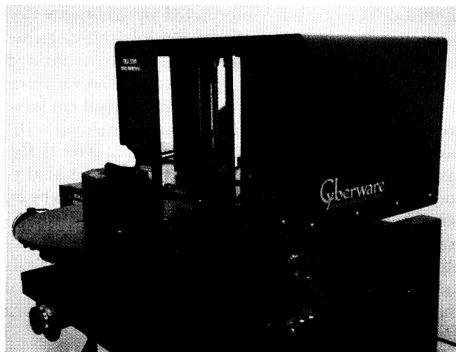
Fig. 2. The Cyberware 3030R-HIREZ high-resolution, monochromatic digitizer (Cyberware Laboratories, Inc., Monterey, California, USA). A white-coloured plaster model is mounted on a blackened wooden block and placed on the circular motion platform. During the scan, the motion platform will swivel and move sideways as the laser pans the plaster model.
