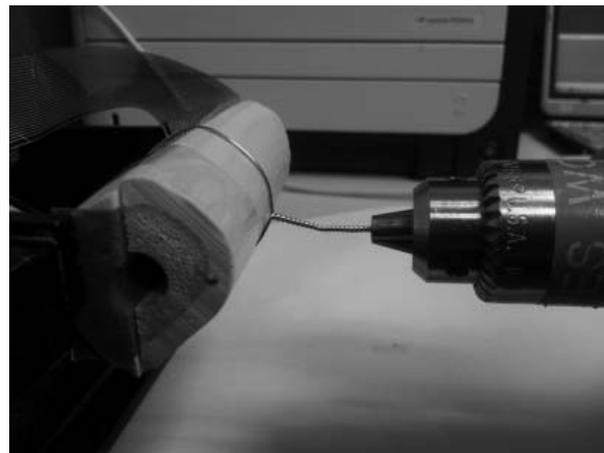
Fig. 2. Each synthetic femur bone specimen was cut into half lengthwise and pressure sensors were placed in between the fragments. The fragments were subsequently compressed via cerclage wiring.
