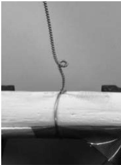
Fig. 3. Secondary coiling of wires.
