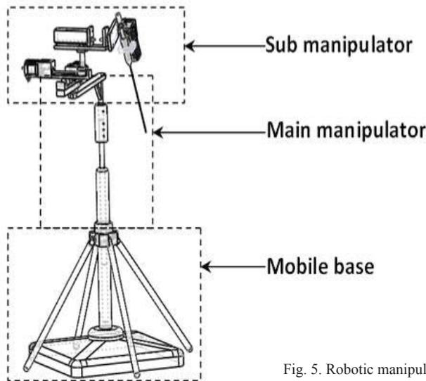
Fig. 5. Robotic manipulator for needle insertion.
