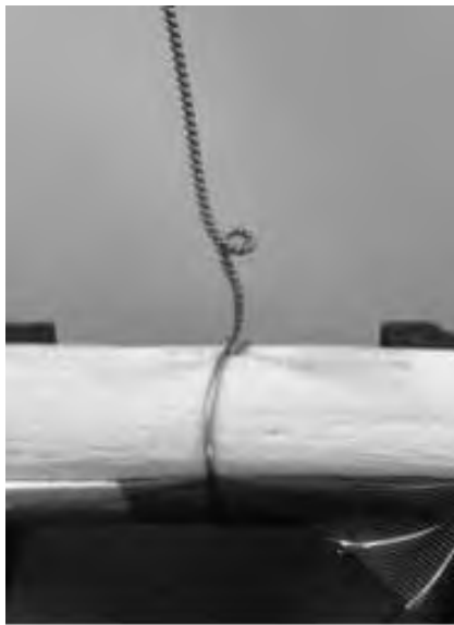
Fig. 3. Secondary coiling of wires.
