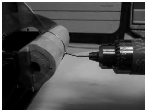
Fig. 2. Each synthetic femur bone specimen was cut into half lengthwise and pressure sensors were placed in between the fragments. The fragments were subsequently compressed via cerclage wiring.
