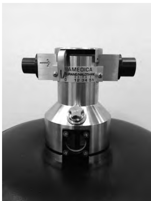
Fig. 1. Diamedica Draw-over Vaporiser (DDV) for isoflurane/halothane. It is a common vaporiser for halothane and isoflurane.
